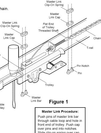
Slide clip-on spring over cap and into notches until both pins are securely locked.
